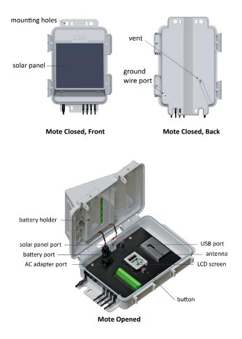
AC Adapter Port: Use this port to plug in an AC adapter (see *Battery Information*).
