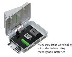
The mote contacts the network once the new batteries are installed. The green LED blinks quickly while the mote searches for a network to join and then blinks slowly while it completes the network registration. Once the mote has finished joining the network, the green LED turns off and the blue LED then blinks indefinitely while the mote is part of the network.
