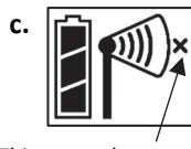
This network connection "x" icon blinks while the repeater completes the registration process, which may take up to five minutes.
