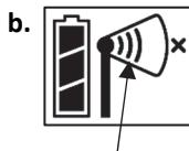
Once a network is found, the icon stops blinking and the bars cycle from left to right.
