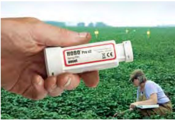
HOBO Pro v2 data loggers are weatherproof loggers that provide high accuracy temperature and relative humidity measurements in a wide range of outdoor environments.
