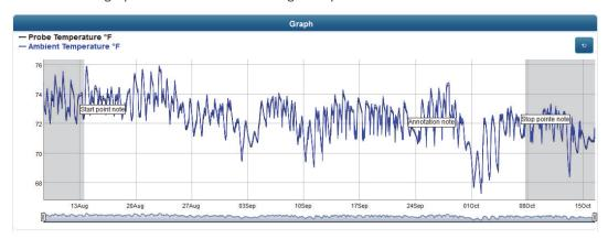
The start and stop date listed in the Configuration Info section change to those selected in the Segmentation Settings, as applicable. The statistics are also recalculated based on the revised total data points remaining in the segmented data.
