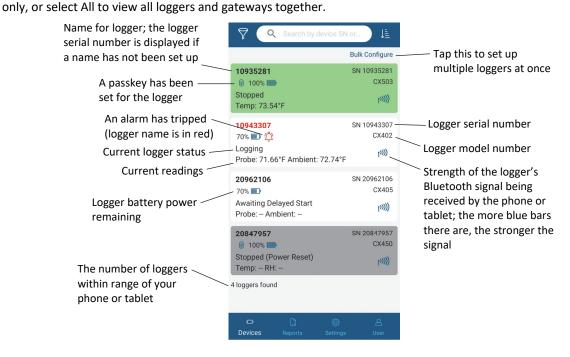
**Note for CX400 loggers:** Probe and sensor readings are displayed as "--" when the logger is stopped. "Error" is displayed if the probe is disconnected from the logger. Probe and sensor readings are updated at a different rate than the logging interval and may not match what is currently displayed on the logger LCD.
