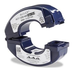
The Accu-CT ACTL-1250 series split-core current transformers provide revenue-grade accuracy with a 0.33333 volt or 1.0 volt AC output.
