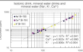
Measurement data of ion chromotography (ppm) \*When measuring Ca2+, we are pretreated in order to match the condition ns of the ion chromatography
