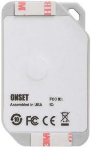
Onset's HOBO MX100 is a low-cost, splash-proof data logger that measures and transmits temperature data wirelessly to mobile devices via Bluetooth Low Energy (BLE) technology.
