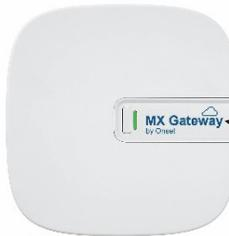
For wall mounting, position the gateway facing the coverage area with the logo oriented as shown
