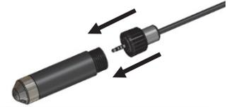
**Important:** Make sure the O-rings on the cable jack end and the cable and sensor mating housing surfaces are clear of any debris. Any contamination of these surfaces can cause leaks that may lead to sensor failure.
