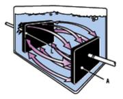
Conductivity can be measured from first principles by using a conductivity cell. This is a box containing a liquid, with two plates, each of area A separated by a distance L.
