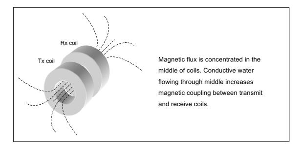
The above diagram shows how the sensor works. Transmit (TX) coil forms a magnetic flux inside the coil pair. Conductive water increases the magnetic coupling which is seen as a transfer of oscillating current in receiver (Rx) coil. The degree of transfer is an indication of water conductivity.
