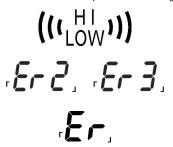
'Hi' or 'Lo' is displayed when the temperature being measured is outside of the settings of HAL and LAL.
