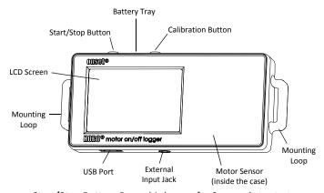
**Start/Stop Button:** Press this button for 3 seconds to start or stop logging data. This requires configuring the logger in HOBOware with a push button start or stop (see *Setting up the Logger*). You can also press this button for 1 second to record an internal event (see *Recording Internal Logger Events*) or to turn the LCD screen on if the option to turn off the LCD has been enabled (see *Setting up the Logger*).
