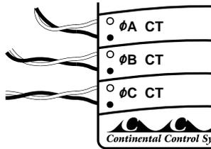
**Note:** Be careful to match the CT to the voltage phases being measured. Make sure the  $\phi A$  CT is measuring the current on the  $\phi A$  conductor, and the same for phases B and C. Use colored labels or tape to identify the wires.
