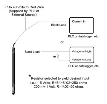
For voltage or battery operated applications, cables should be kept less than 1000 feet in length due to capacitance and impedance of the cable. Also, the linear, finite resistance associated with the additional length of the cable should be taken into consideration.
