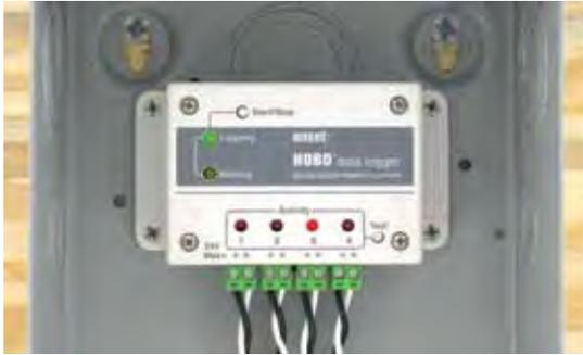
The HOBO UX120 4-Channel Pulse Input Data Logger is a highly versatile, 4-channel energy data logger that combines the functionality of four separate energy loggers into one compact unit. It enables energy management professionals – from energy auditors to building commissioners – to easily track building energy consumption, equipment runtimes, and water and gas flow rates.
